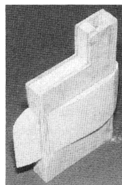
18. The assembled and shaped float strut. The raised portion has been deleted from the drawings.
