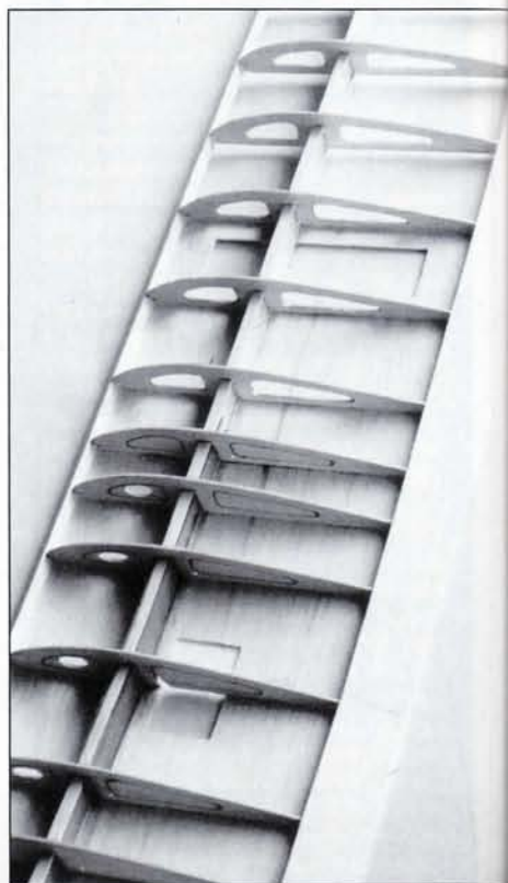
Basic wing structure. Notice the cutout for the aileron servo in the center section of lower skin, and cutout for the float well midway to the tip.
