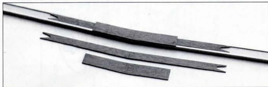
Wing spar center section with one spar doubler and dihedral brace in place.
