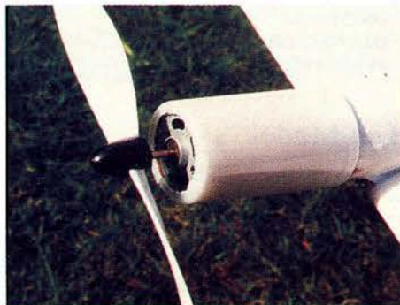
▲ Engine cowling is a 35mm plastic film can.
