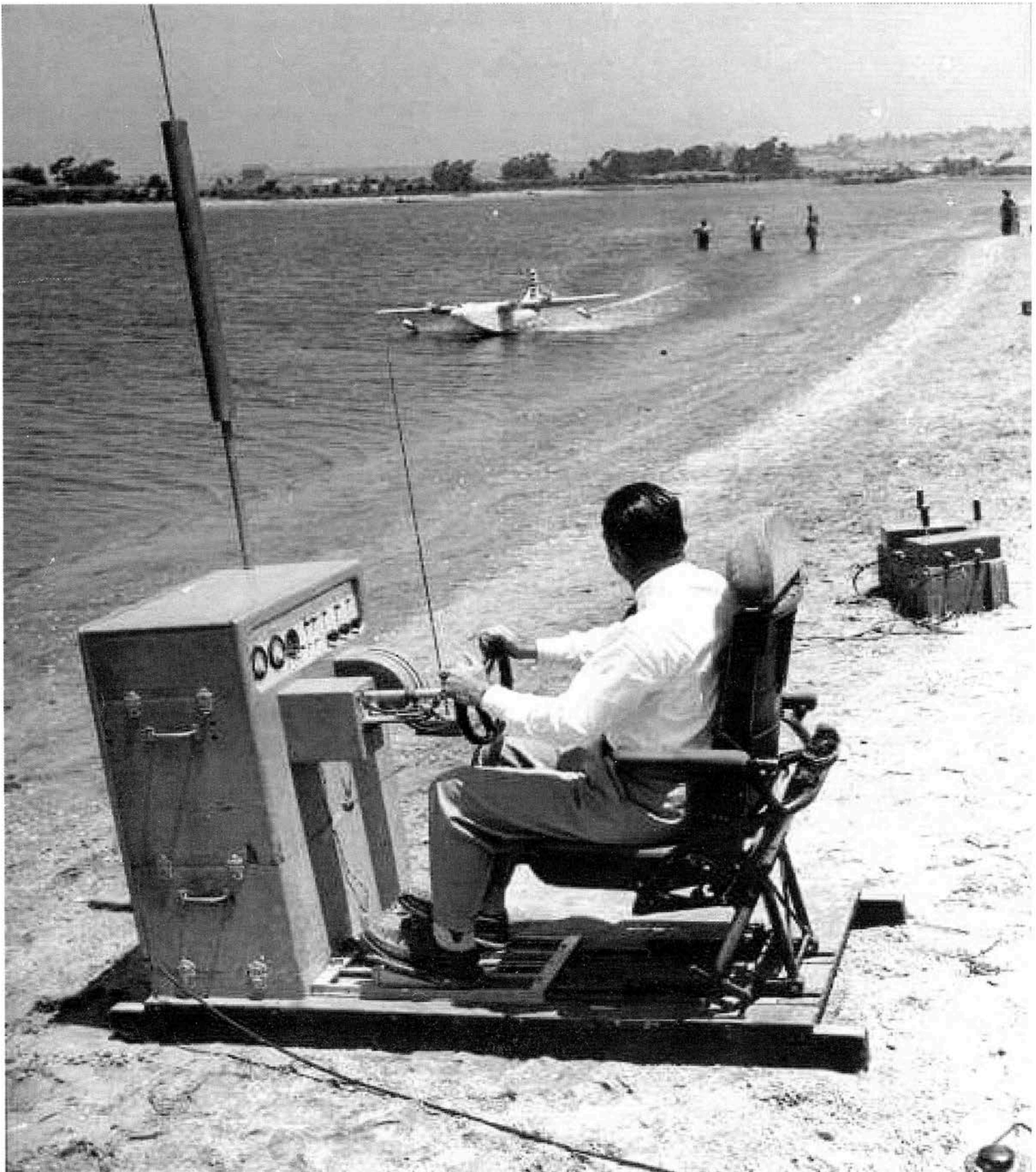
Howard Hughes test flying a scale test model of the Hughes H-4 Hercules (better known as the Spruce Goose, a name that Hughes hated).
