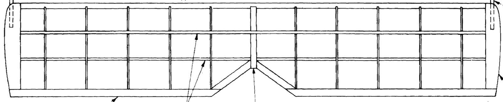
EMBED ALUM. TUBE BRACES IN SOFT BALSA TIPS & HOT STUFF
