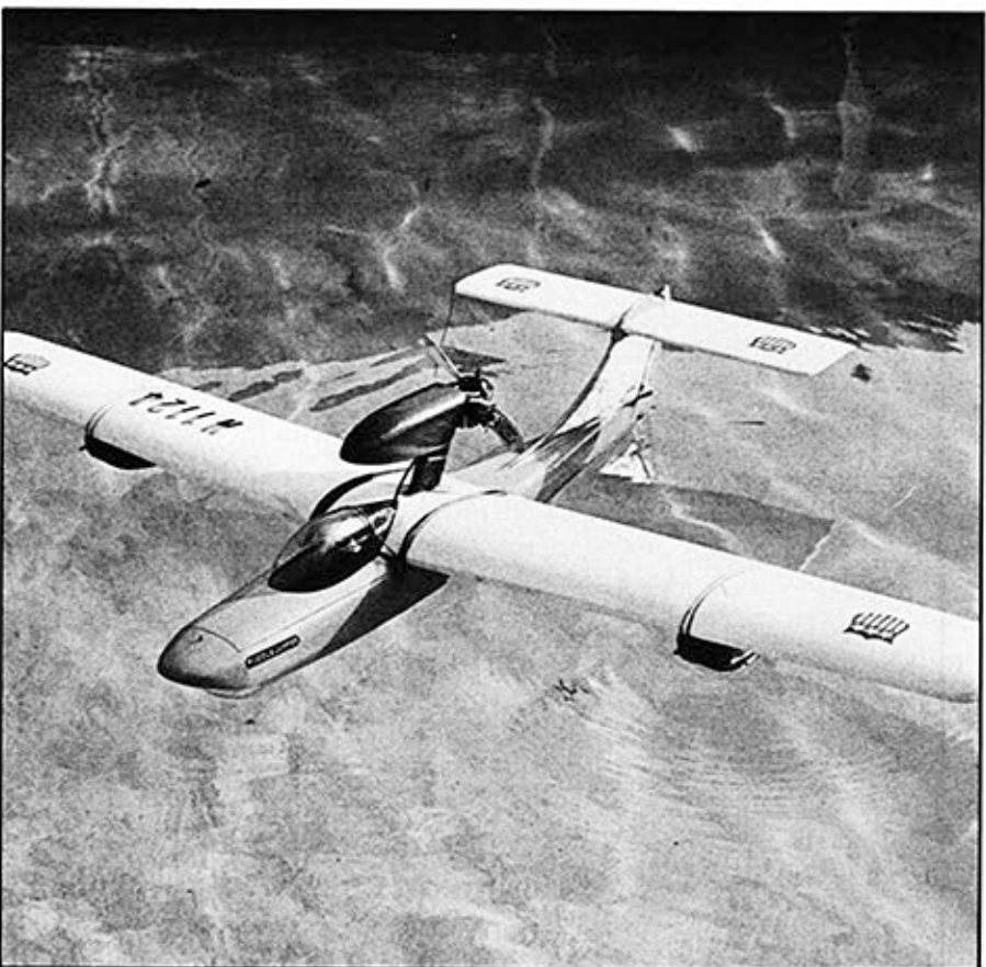
ABOVE: The Puddlejumper is as versatile as it is quick to build. Here it is shown in its landplane configuration. The landing gear can be quickly removed to make it a -----
