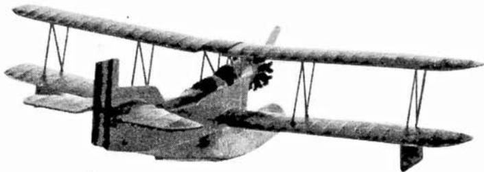
*A complete change from the usual run-of-the-mill scale subjects, this Loening will fly equally well over grass or water. Engine and prop are protected by the long hull and construction allows fully "crash proof" knock-off wing fixing. Full size copies of the 1/6th scale plan opposite are available price 7/6 post free from AEROMODELLER plans Service. Quote Plan No. FSP 650 when ordering*
