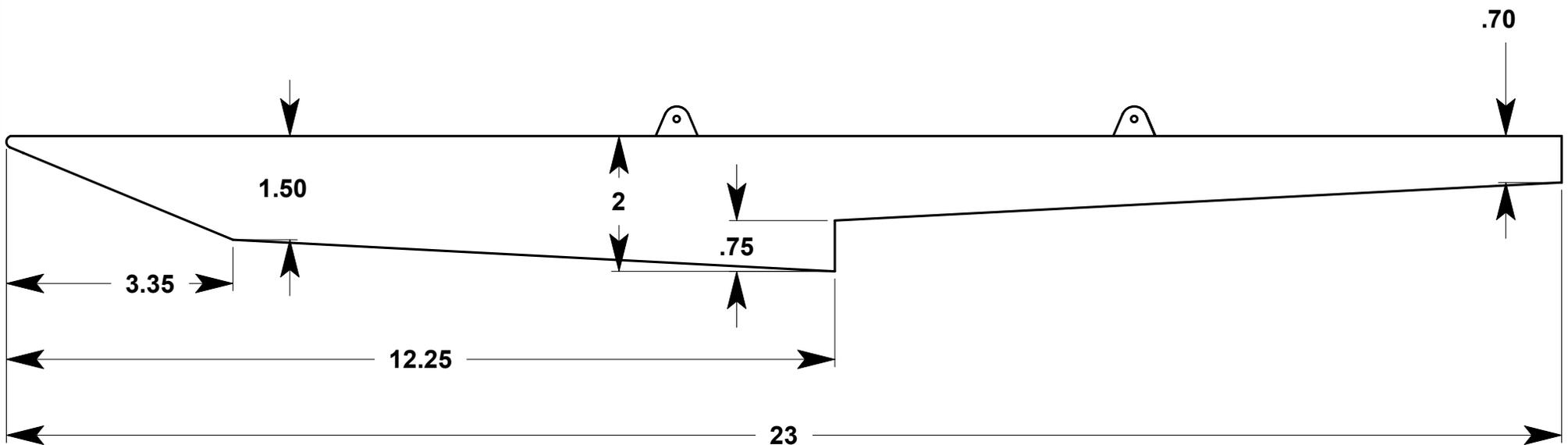
**MAKE THE REAR FLOAT SUPPORT 1/4" SHORTER IN HEIGHT THAN THE MAIN LANDING GEAR. THIS PROVIDES A POSITIVE WING INCIDENCE WHEN THE MODEL IS MOVING THROUGH THE WATER.**
