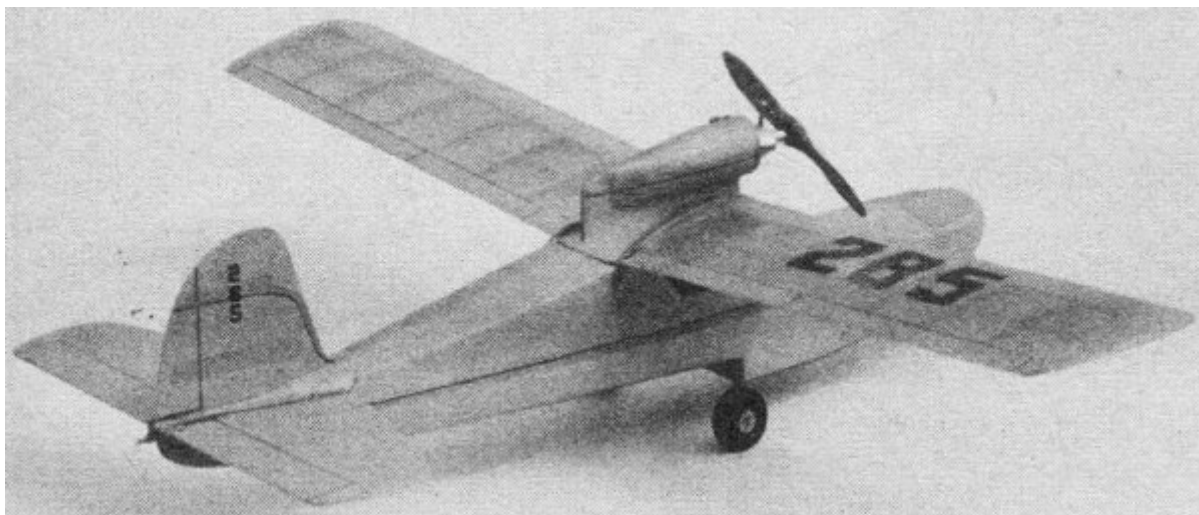
Lower engine mounting and fairly wide hull enables ship to get off water without help of troublesome sponsoons or tip floats. Weight is 8 ounces.
